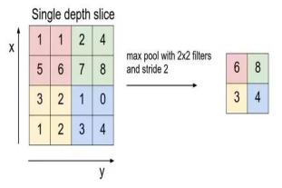
The dimensional of the pooling layer of an input image is 32x32x10. The result of this pooling layer will be in 16x16x10 feature map. In the output the wi dth and height of the feature map are
