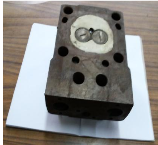
Figure 1- Photographic view of ceramic coated cylinder head
