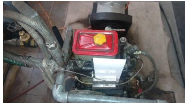
Fig. 3 Installation of Magnetizer Set Up on the fuel line.
