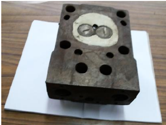
Fig.1 Photographic view of ceramic coated cylinder head
