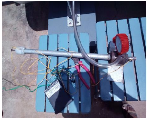
Figure- 5.1. 54.61cm tube length vortex tube refrigerator
