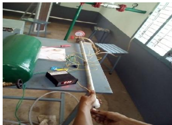
Figure- 5.2.102.87cm tube length vortex tube refrigerator
