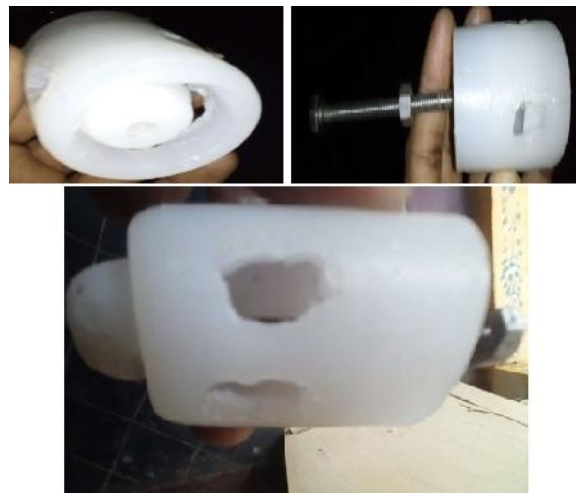
Figure- 4.7 Control Plug for flow control
