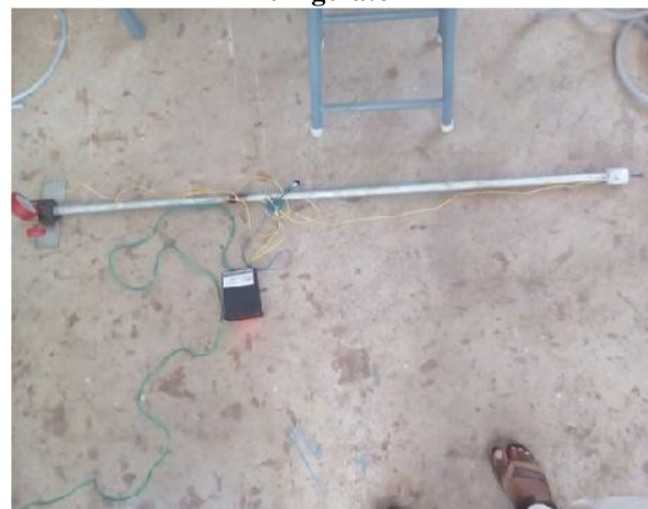
Figure- 5.3.119.38 cm tube length vortex tube refrigerator
