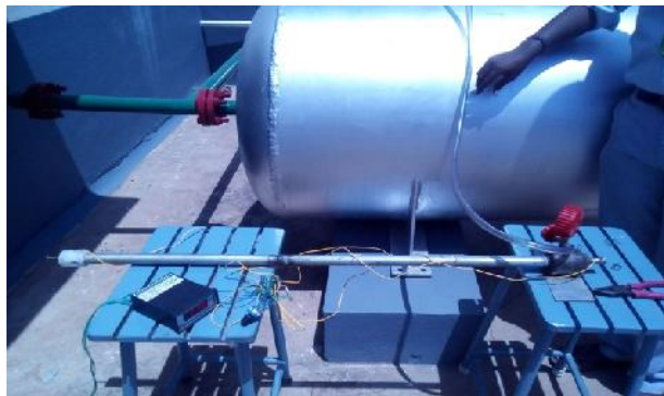
Figure- 5.5 Complete setup of Vortex Tube Refrigeration system with compressor connection
