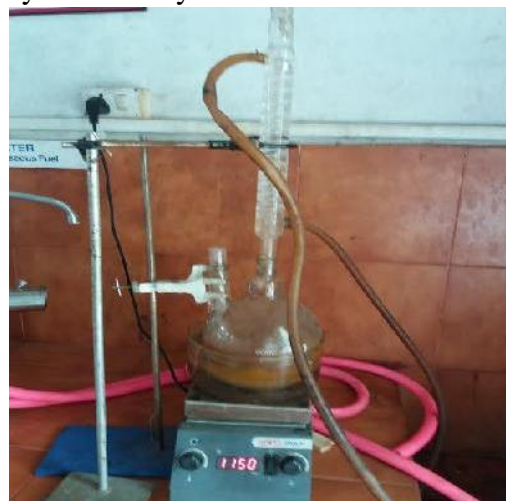
Figure: Transesterification Equipment
