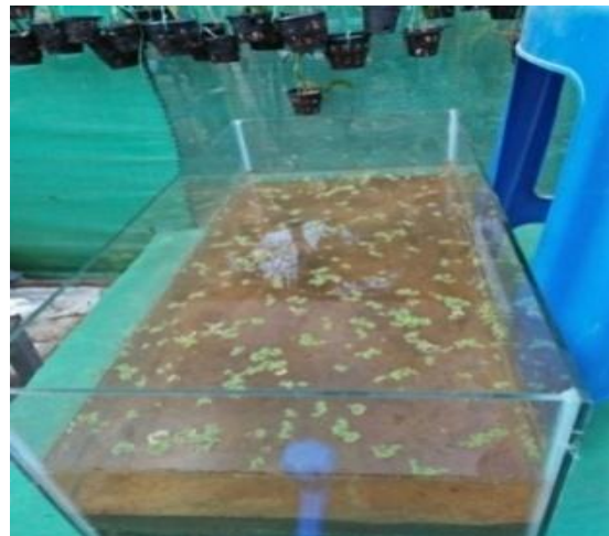
Figure - 3 Azolla pinnata planted in dairy waste water wetland unit (Before treatment)
