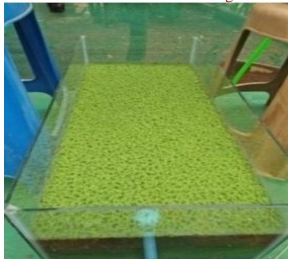
Figure - 2 Azolla pinnata plant growth in dairy waste water wetland unit (After treatment)
