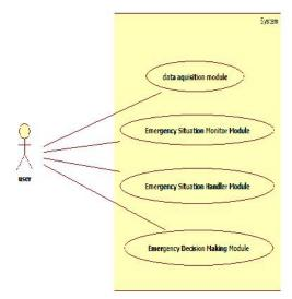
The use case diagram is vigorous in nature there should be some internal or external factors to make interactions. These internal and external agents are known as actors. Use case diagram consists of actors, use cases and their relationships. The diagram is used to model the sys-subsystem of an application. Single use case diagram captures a particular functionality of a system. So to model the entire system various use case diagrams are used.
