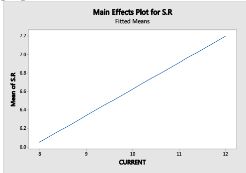
Figure. 4 Main effects plot for S.R for H-13 metal
