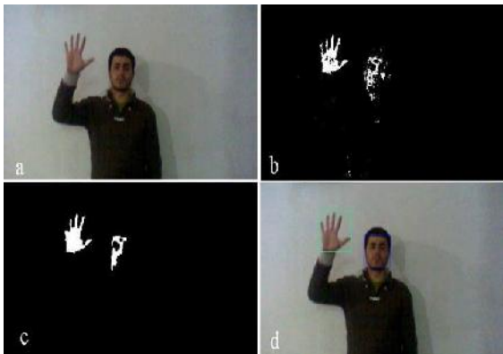
Figure 1. (a) Entrance image (b) Detected skin region (c) result of mathematical morphology (d) detected face and hand region
