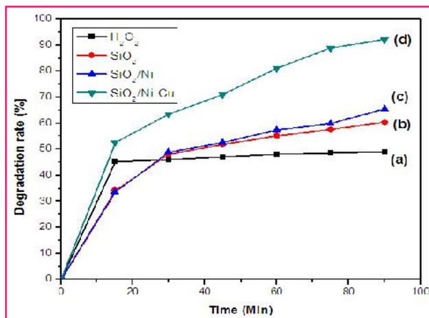
Figure 4- The effect of ((a) H<sub>2</sub>O<sub>2</sub> and H<sub>2</sub>O<sub>2</sub> mediated (b) SiO<sub>2</sub> nanoparticles, (c) SiO<sub>2</sub>/Ni and (d) SiO<sub>2</sub>/Ni-Cu on the degradation of MB dye as a function of time
