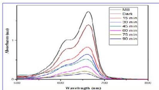
Figure 3- UV-Vis spectra of MB degradation process influenced by  $SiO_2/Ni-Cu$  observed at a time interval of 15 min
