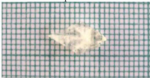
Figure 1- Photograph of Pure BTCC crystals
