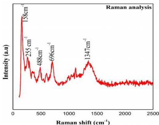
Figure 3- Raman analysis of  $\text{Li}_2\text{FeSiO}_4$  prepared sample
