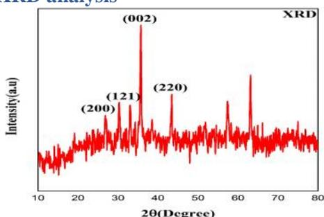
Figure 1 - XRD pattern of  $\text{Li}_2\text{FeSiO}_4$  prepared sample
