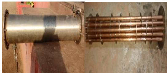
Figure.1 Actual Photograph of Shell and tube along with baffle arrangement.
