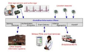
Ubiquitous Monitoring Environment for Wearable and Implanted Sensors: It shows the aim of having aUbiMon for wearable and implantable sensors is to provide continuous management of patients under their natural physiological states. The system is mainly used for collecting, gathering and analyzing data from number of sensors
